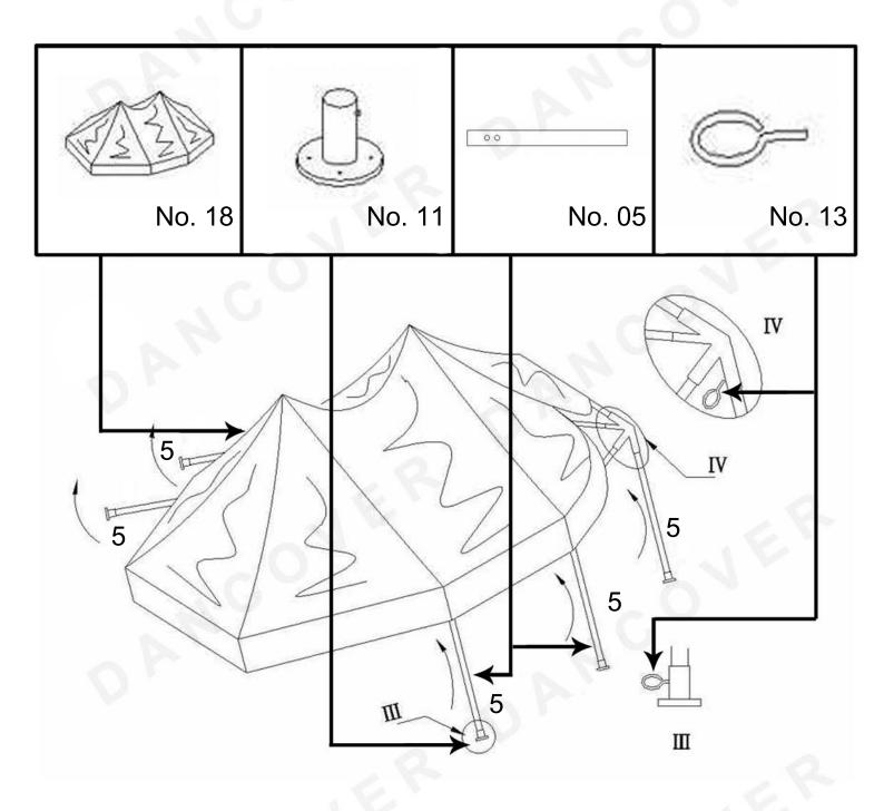
**Step 5:** Put the roofcover on the frame.
