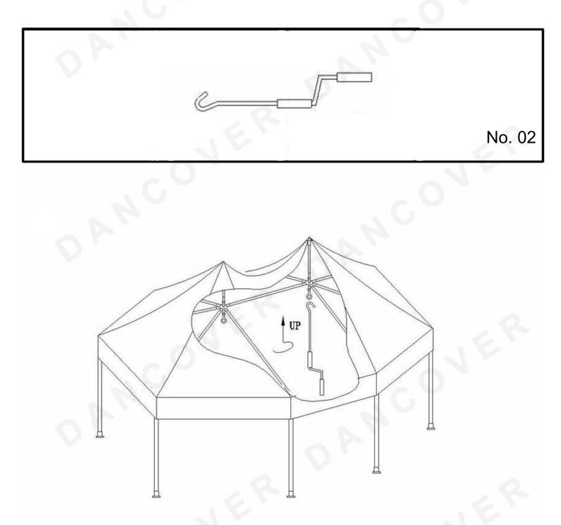
**Step 11:** Tighten the Roofcover using No. 02 as shown above.
